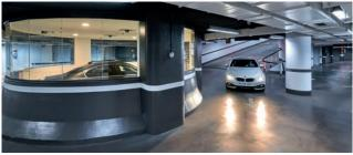
A separate driving lane is provided for entering and for exiting the system. Right before transiting through the entrance barrier, the user is notified exactly which one of the five car transfer stations has to be accessed directly. As soon as the barrier opens up, thanks to cleverly automated parking guidance systems the driver comfortably reaches the designated transfer area. Seamless parking operations are thus ensured at all times.
