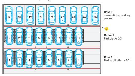
2 Light barriers must be provided for multi-row arrangements compliant to DIN EN 14010.
