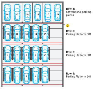
2 Light barriers must be provided for multi-row arrangements compliant to DIN EN 14010.
