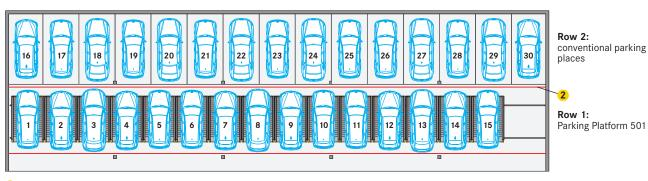
2 If the rail length is more than 30 m, light barriers compliant to DIN EN 14010 must be provided.
