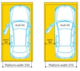
Depending on the vehicle model and the parking position of the vehicle on the platform, the space for opening the door varies. For comfortable conditions for getting in and out of the car, we recommend platform widths of at least 270 cm.
